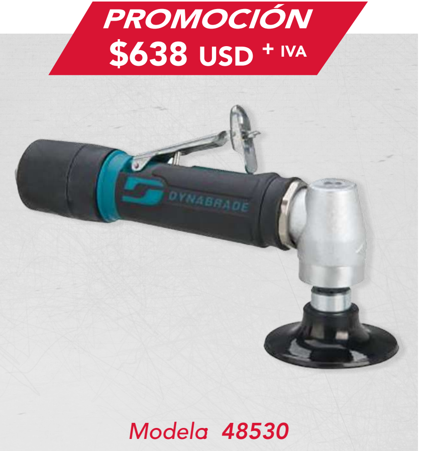
3" (76 mm) Dia. Right Angle Disc Sander .4 hp, 12,000 RPM, Geared, Extended Rear Exhaust, Locking-Type Female Pad.
